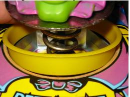
It is not possible to work all the way round due to the rigidity of the protector, Instead you should be able to get a minimum of 2/3 of the lip on the protector into the hole.
