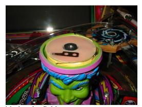
This will aid in aligning the top plate level with the playfield.
