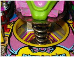
I suggest that after pushing into place, you rotate the ring to seat it and also to position any kink evidence to one side (it will naturally unkink over a short period of time). If you do notice any wear during operation, it is possible to rotate the protector to a new point thus prolonging the life of the protector.
